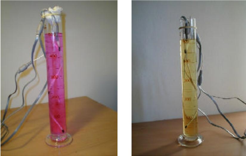
Fig. 1: The first cylinder is filled with alcohol and the second with oil; three temperature probes can be seen in each one.
