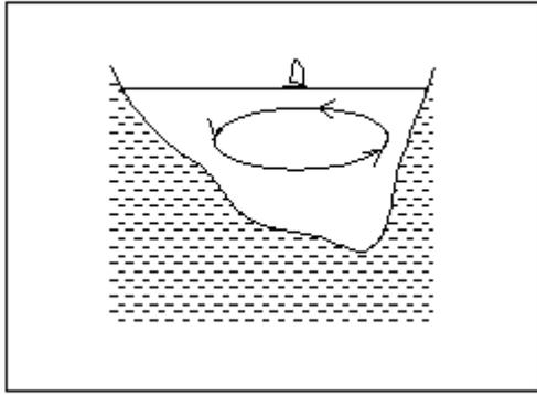
Fig. 4: Below 4°C the water mass involved in the convection currents becomes smaller.
