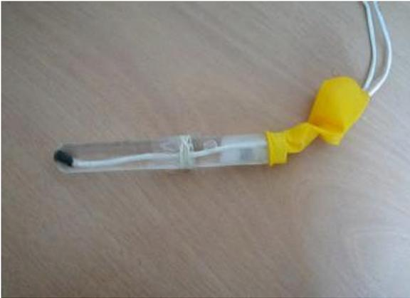
Figure 3: test tube at the end of the experiment. The layer of ice in the upper part is visible; the elastic bands are placed at mid tube, the probes are at the bottom and inside the ice layer; the plastic balloon is used to avoid “pollution” of the lake with salt water.
