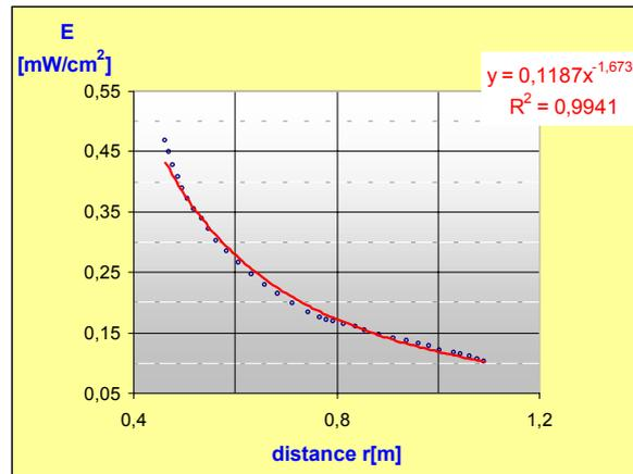
Fig.24. Irradiance vs distance. Experimental data and power type approximation
