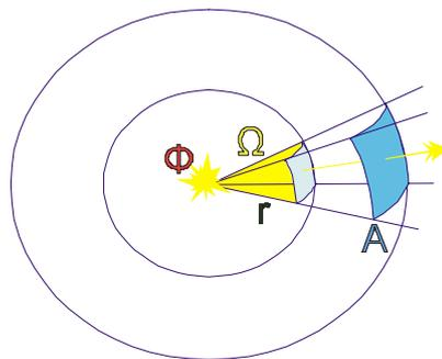
Fig.1. Radiant flux  $\Phi$  and radiant intensity  $I$
