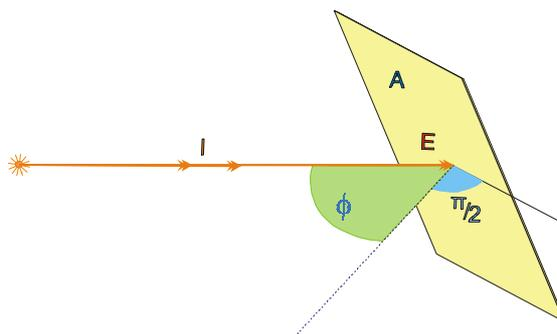
Fig. 3. Irradiance  $E$  at the inclined plane
