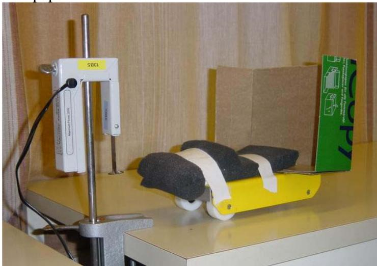
It is convenient to use a table with a length of about one and a half meter for the experiment. The force sensor must be mounted firmly for example at the edge of the table, and its height adjusted so that the collision takes place as intended. Put the CBR behind the cart and about half a meter from the start position of the cart about one meter from the force probe.
