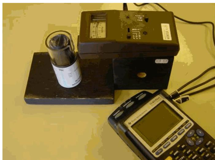
Connect the Radiation Monitor to the calculator. Be sure that you use the Dig/Sonic input.
