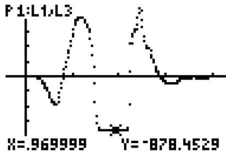
We see that the net force is 0 at the beginning and at the times 0.40 s, 0.73 s and 1.12 s. These values can be found using TRACE on the graph.
