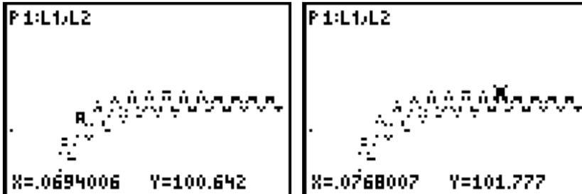
To get better accuracy we have chosen two points at a time distance more than one period apart. The choice is seven complete oscillations. The length of the time interval between these is  $0.0768 \text{ s} - 0.0694 \text{ s} = 0.0074 \text{ s}$ .
