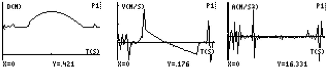
The central part of the position plot is not symmetrical thus revealing that acceleration has not the same value while the toy car is going uphill and downhill. Still it may be important to perform a linear regression selecting all the data at a time to stress that as a first approximation the acceleration value should be the same.
